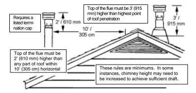
To achieve a stable draft, the total flue height required (from the appliance to termination) is 12 to 15 feet minimum.
